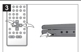
Close the disc tray. After loading, the menu screen of the DVD should appear. Use the Navigation  $(\blacktriangleleft, \blacktriangleright, \blacktriangle, \blacktriangledown)$  buttons ① to select the desired option and press the PLAY/ENTER button ② to select it. Adjust the VOLUME control ③ as desired.
